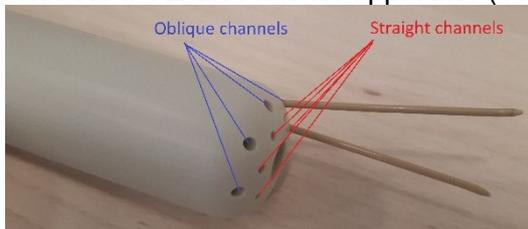
1a.) New cylinder with combined straight and oblique channels (old standard: only oblique)
