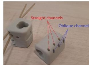
1b.) New ovoids with combined straight and oblique channels (old standard: only straight)
