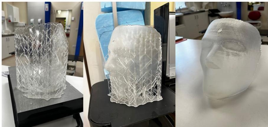
*Figure 1: Shell after print (left), after washing/curing (middle) and after removal of supports (right).*
