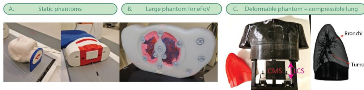
Figure 1: An overview of the manufactured phantoms in the physics research division for brachytherapy dosimetry verification (A), a large breast phantom used in eFoV evaluation (B) and dynamic phantom, containing a motion platform (A) and a deformable thorax phantom (C) to simulate patient breathing
