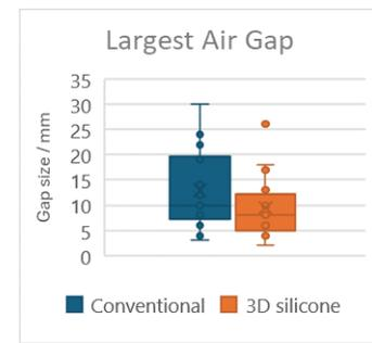
33/35 silicone and 20/20 TPU boluses passed QA with geometric deviation <0.5mm and density within 30HU of baseline. Silicone failures arose from air bubbles causing shape changes and inhomogeneity, but neither deviation significantly altered planned dose distributions.
