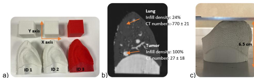
**Figure 1.** a) 3D-Printed cubes & miniature lungs. b) CT slice of a sample 2 and c) a demonstration of the compression range of sample 2, the original height at 11 cm and compressed height at 6.5 cm.
