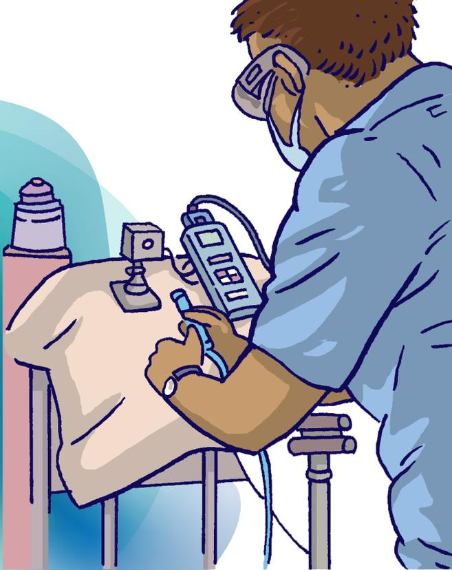
Laser output measurements being taken using a thermopile sensor and a power and energy meter
