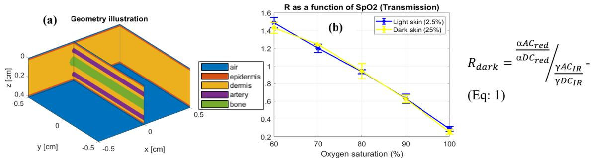
Figure 1: a) Geometry of the 4-layer Tissue model. b) SpO<sub>2</sub> vs R curves for light and dark skin. Note: In Eq1,  $\alpha$  and  $\gamma$  represent the attenuation factors due to skin colour at red and IR wavelengths.
