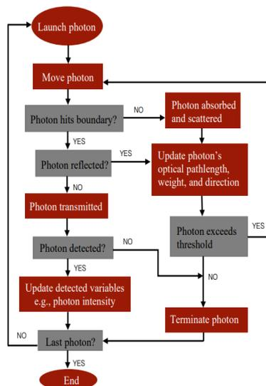
Fig. 1. Monte Carlo algorithm flowchart
