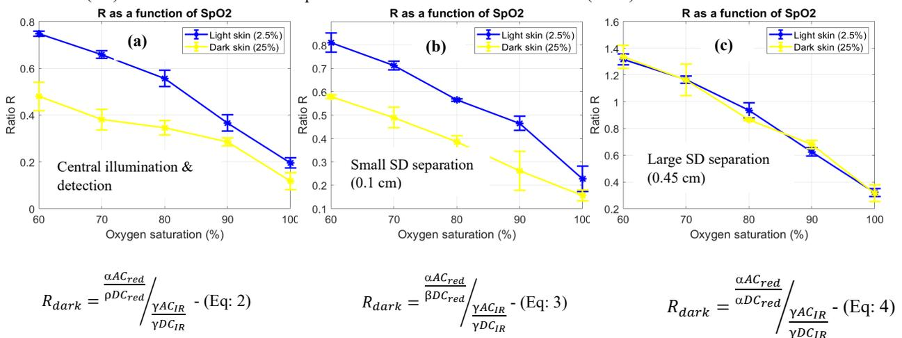
Figure 2: SpO<sub>2</sub> vs R curves shown for a) Central illumination and detection. b) small SD separation (0.1cm). c) Large SD separation (0.45 cm). Note:  $\alpha$ ,  $\gamma$ ,  $\rho$ , and  $\beta$  all represent different attenuation factors due to skin colour at red and IR wavelengths (*Attenuation factors  $\rho > \beta > \alpha$* ).
