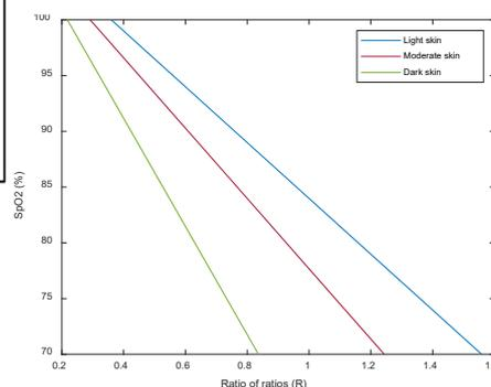
Fig. 2. Simulated calibration curves for light, moderate, and dark skin
