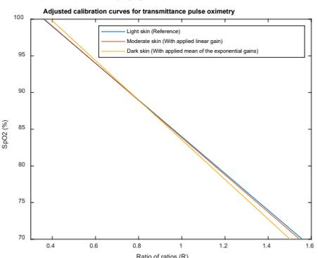
Fig. 3. Adjusted calibration curves for moderate and dark skin
