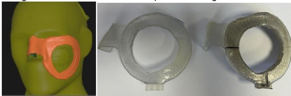
Figure 1: Creation of the mask in the TPS (Raystation), printed MED610 mask and Cerrobend-filled mask.
